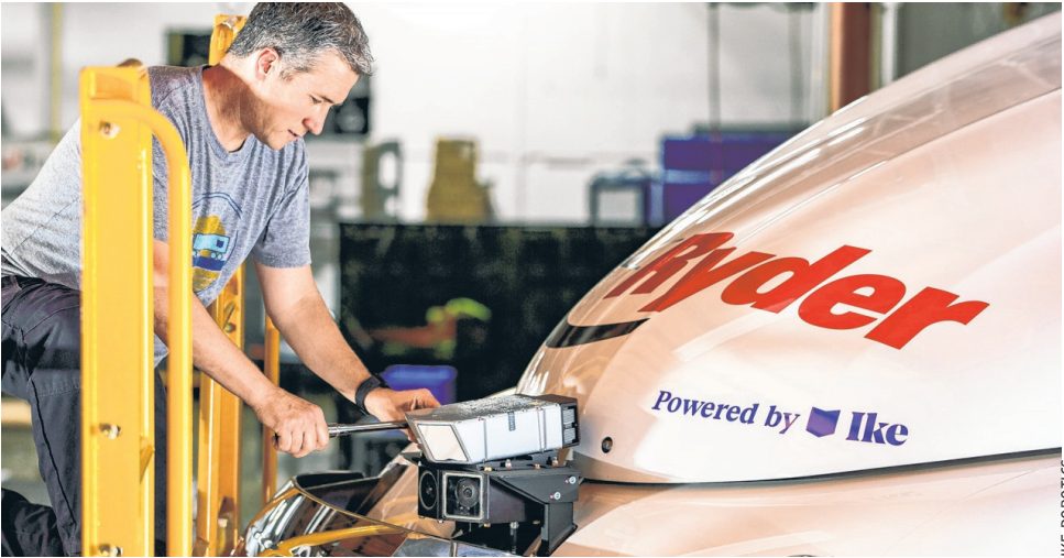
An Ike Robotics technician works on the sensor of a Ryder truck to make the vehicle self-driving.
